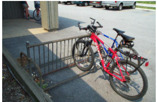
Another standard design, wheel only. These racks were designed in the days when most bikes were sold with wheels bolted to the frame, and a simple loop through the wheel rim was secure enough to prevent theft in most cases. Note the blue bike parked alongside the rack to allow for frame locking.
