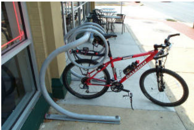
Downtown Newark, next to Starbucks. This is well designed for locking the frame of the bike, a wheel, and anything else higher up, such as the saddle.
