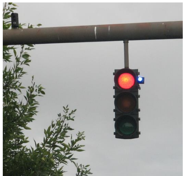
Photo 5: Blue Light Detector Feedback Device (Source: FHWA Separated Bike Lane Planning and Design Guide)
