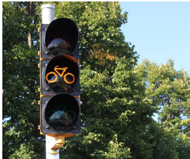
Photo 3: Bicycle Signal Head (Source: NACTO)
